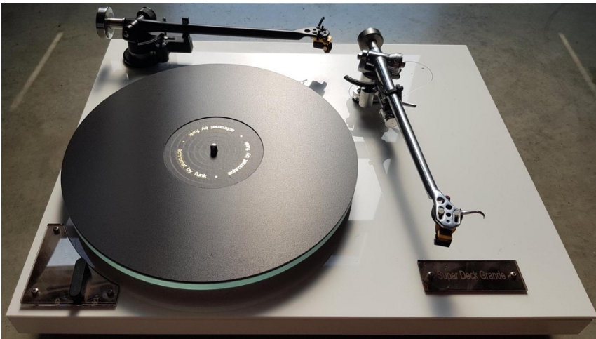
Old RB 300 at rear and RB3000 to the right.
